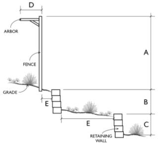
If measurement "E" is less than 24 inches, the fence and retaining walls are measured together (e.g., A+B=Height).
