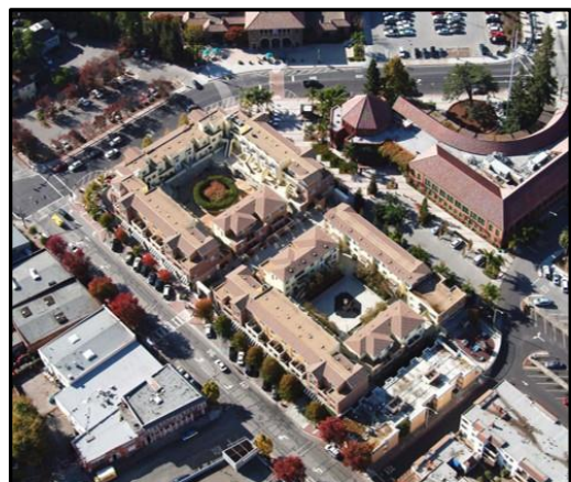
City Center Plaza in Redwood City, California, is a mixed-use affordable housing development. It has 81 units with a density of 46 du/ac.
