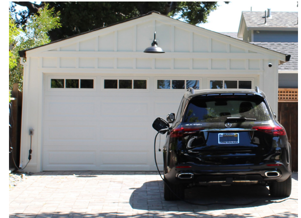
Figure 2.21.1: Lights on the building facade shall fully shielded and directed downward onto the building facade and onto paving of entrance areas.
